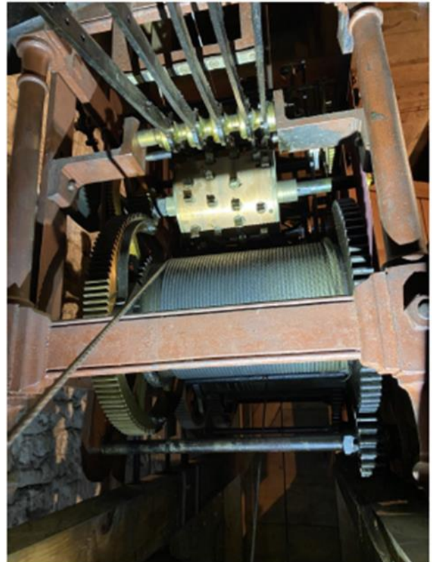
Chime-side view. Note chime pin-barrel at second level.
