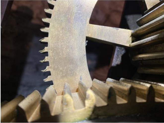
Wear to tooth profile, quarter-chime second wheel. Photo: RG
